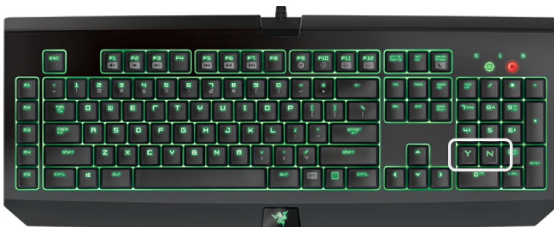
Figure 1. Keyboard with Yes/No Key. A keyboard for behavioral and EEG experiments with stick-on 'Y' and 'N' labels on neighboring keys to indicate 'Yes' and 'No' responses. Please click here to view a larger version of this figure.
