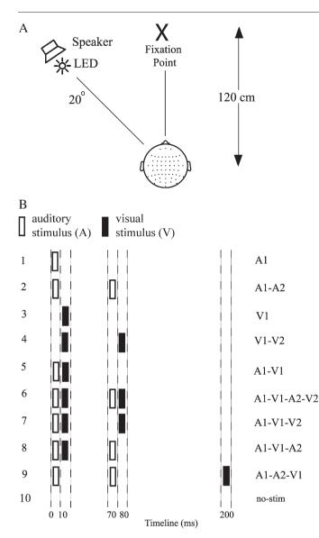
Fig. 7 – Overview of experimental design. [A] Schematic diagram of experimental set-up. [B] Listing of the ten different stimulus configurations, which were presented in random order. Abscissa indicates times of occurrence of auditory (open bars) and visual (solid bars) stimuli. Auditory (A) and visual (V) stimuli are labeled 1 or 2 to designate their first or second occurrence in each configuration (adapted from Mishra et al., 2007).
